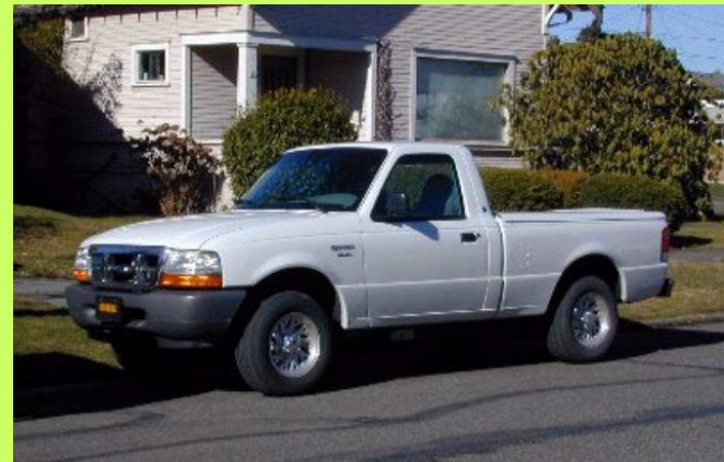
Ford Ranger EV: 82 mile range, 9 hour charge time with NiMH batteries
