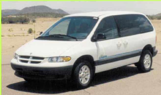
Chrysler EPIC (Caravan EV): 79 mile range, 9 hour charge time with NiMH batteries
