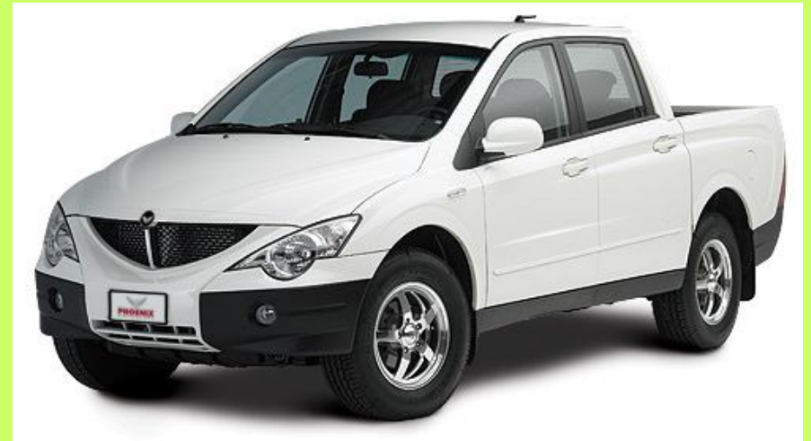
Phoenix Motorcars SUT: 130 mile range, 10 minute charge time with Lithium Ion batteries
