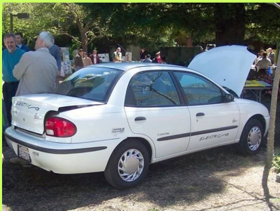
Solectria Force (Chevrolet Metro EV): 84 mile range, 9 hour charge time with NiMH batteries
