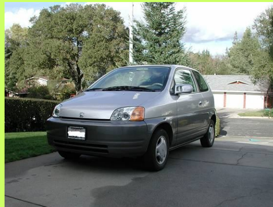
Honda EV Plus: 80 mile range, 8 hour charge time with NiMH batteries
