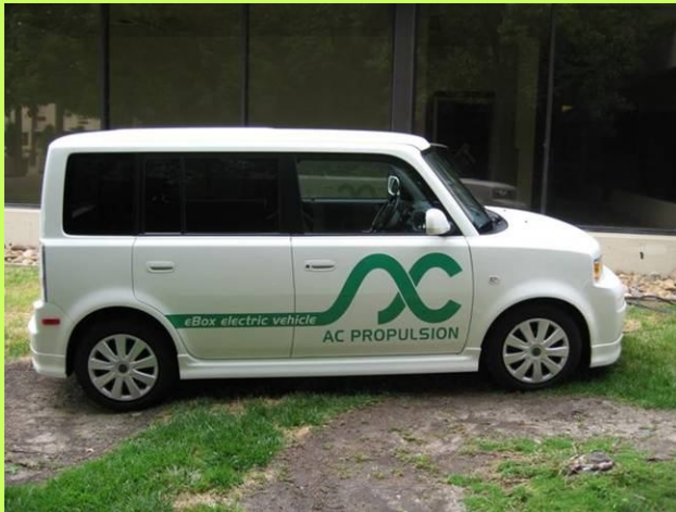
AC Propulsion eBox (Toyota Scion xB EV): 120 mile range, 2 hour charge time with Lithium Ion batteries; $55K plus Scion xB
